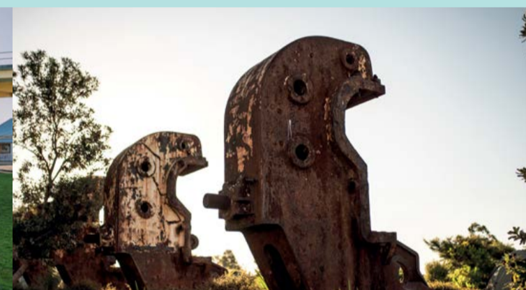
Remnants of a 1920 Hugh Smith Plate Bending Machine
